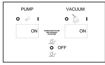
Turn on Pump and Vacuum Switch. Note: Be sure intermittent/continuous switch is in center (off) position and brush is in storage position.
